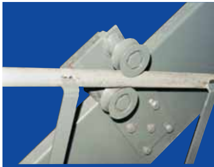
Handrail Roller Guides
